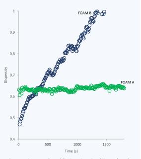
Coarsening or Oswald ripening is driven by the pressure gradient between different sized bubbles and lead the gas to move from smaller bubbles (higher gas pressure) to larger bubbles (lower pressure).
